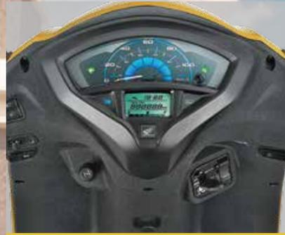
**DIGITAL ANALOG METER WITH ECO SPEED INDICATOR<sup>^</sup>**
