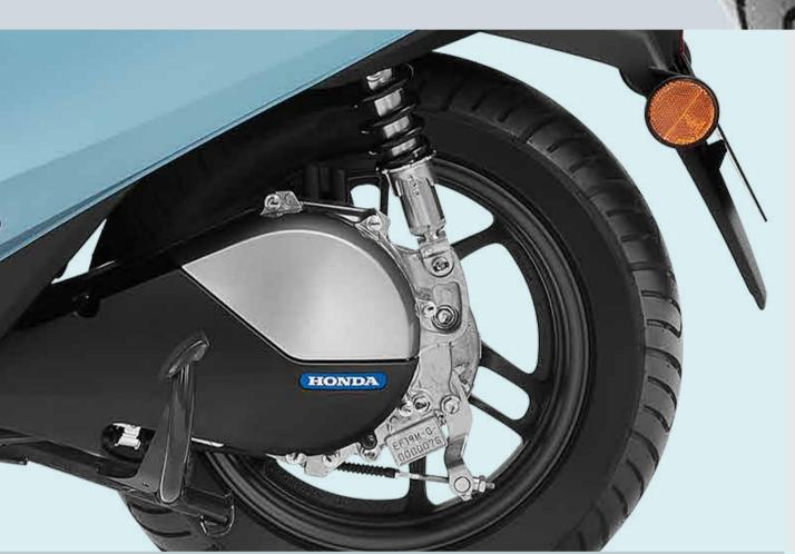
Integrated frame and power unit Exclusively designed for swappable battery to enhance structure, stability, and rigidity of vehicle.
