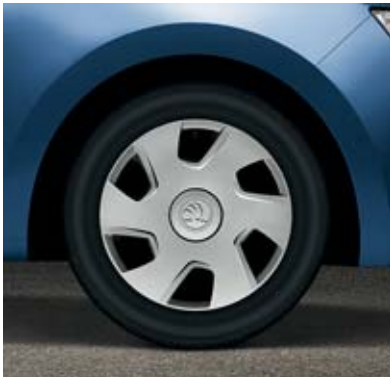
6.0J x 15" steel wheels for 185/60 R15 tyres with Dakar hub covers
