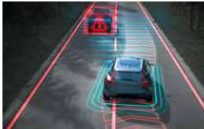
Oncoming Mitigation by Braking A Volvo Cars safety world first, this innovation can detect vehicles heading towards you on the wrong side of the road. If a collision can't be avoided, it can brake your car automatically and tighten the optional prepared front safety belts in order to help reduce the effect of a collision.
