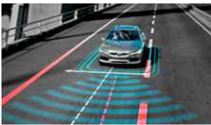
Lane Keeping Aid The Lane Keeping Aid can gently help steer your car back into its lane if it senses you are about to inadvertently cross into a different lane. If this is not enough or if you keep steering across the lane markings, you'll be alerted with vibrations in the steering wheel.
