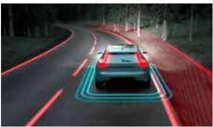
Run-off road Mitigation Stay safely on the road with this Volvo Cars safety innovation. If Run-off road Mitigation detects you're about to leave the road unintentionally, it can provide steering input and, if necessary, brake support to help guide you back on track.
