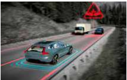
Oncoming Lane Mitigation If you drift across the lane markings and into the path of an oncoming vehicle, your car can alert you and gently steer you back onto the correct path. This system does this using automatic steering assistance, helping you to avoid collisions with oncoming vehicles.
