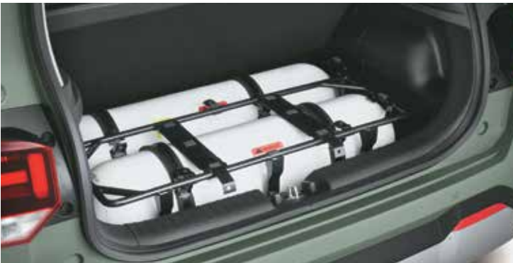
Company fitted dual cylinder CNG
