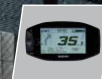
MULTI-FUNCTION DIGITAL METER It displays Digital Clock, Fuel Gauge and Oil Change Indicator, etc.
