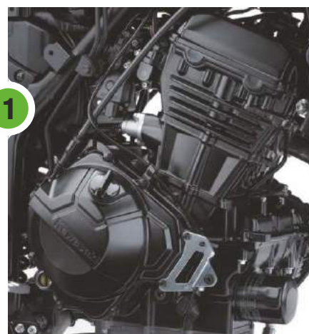
296 cm 3 39PS Fuel Injected Parallel Twin Engine
