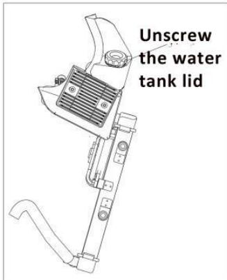
Figure 33 Adding coolant
