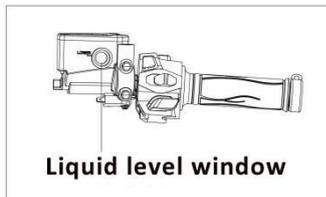
Adjust the placement posture of the vehicle so that the brake fluid in the brake fluid is in a horizontal position, and check the brake fluid level through the fluid level window. (Figure 26)
