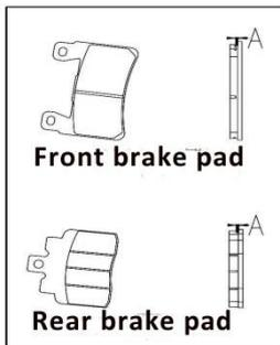
Check the minimum thickness of the brake pads (A).
