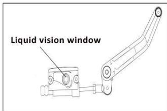
Adjust the placement posture of the vehicle so that the brake fluid in the brake fluid is in a horizontal position, and check the brake fluid level through the fluid level window.
