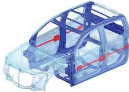
**Cross-car front beam and side-door intrusion beams**
