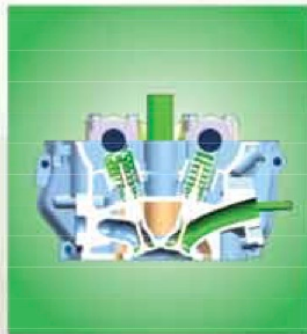
Special material Valve Seats for better durability
