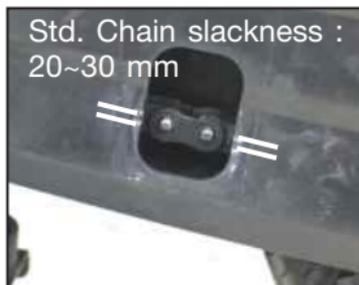
Drive chain must be cleaned & lubricated as per periodic maintenance schedule.
