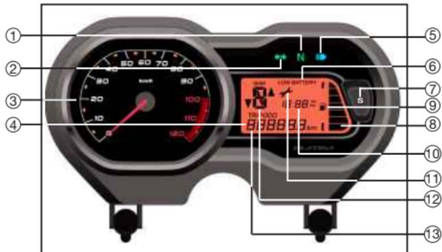
1. **Neutral Indicator** : When the transmission is in Neutral & Ignition switch 'ON', the Neutral indicator will get 'ON'.
